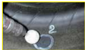
3 Buff the inner liner without forcing.
