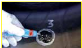
4 Spread the rubber solution over the buffed surface. Leave to dry, 5 min.
