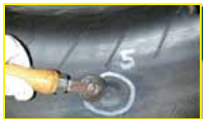
8 Roll the head of the PRP, beginning at the centre and moving outwards.
