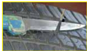
9 Cut off the part which juts out on the outside, without pulling on the body of the PRP.
